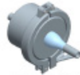
25mm SEGMENT HOLDER FILTER HOUSING SCALE 1:2
